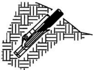
4. DRIVE ANCHOR TO PROPER DEPTH
