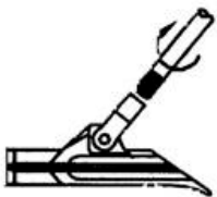
1. THREAD ANCHOR ROD INTO MANTA RAY
